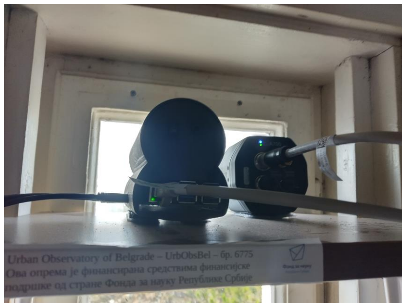
Figure 6. The FLIR A700 infrared camera (on the right) and the HSI detector (on the left) mounted at the Tower of the Astronomical Observatory of Belgrade.
