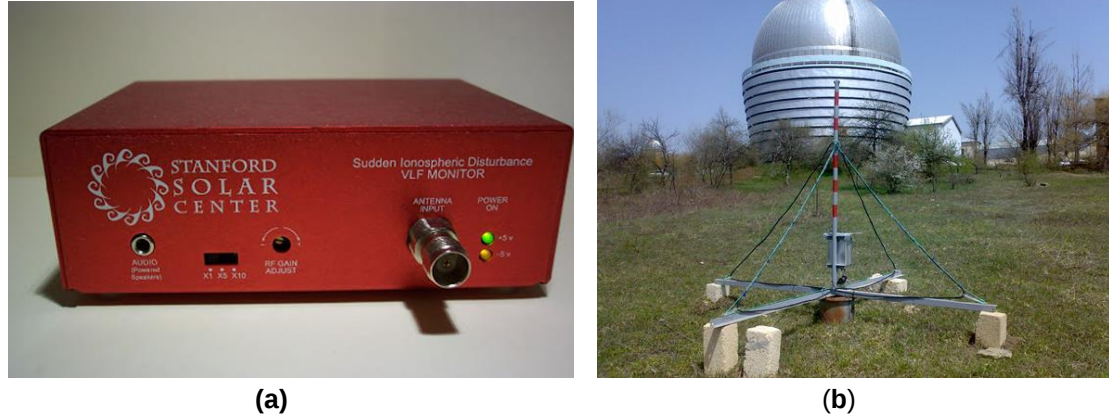
Figure 2. (a) AWESOME receiver and (b) VLF antenna
